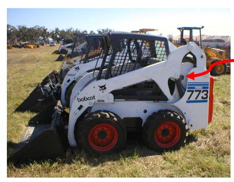
Image of a similar Bobcat 773-T. PIN plate is located on the left side, inset from the loader boom and hydraulic cylinder
